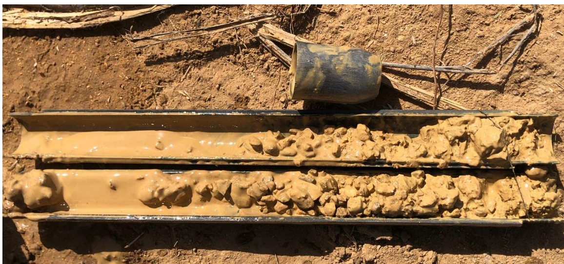
Figure A-3: Soil sample in split spoon sampler
