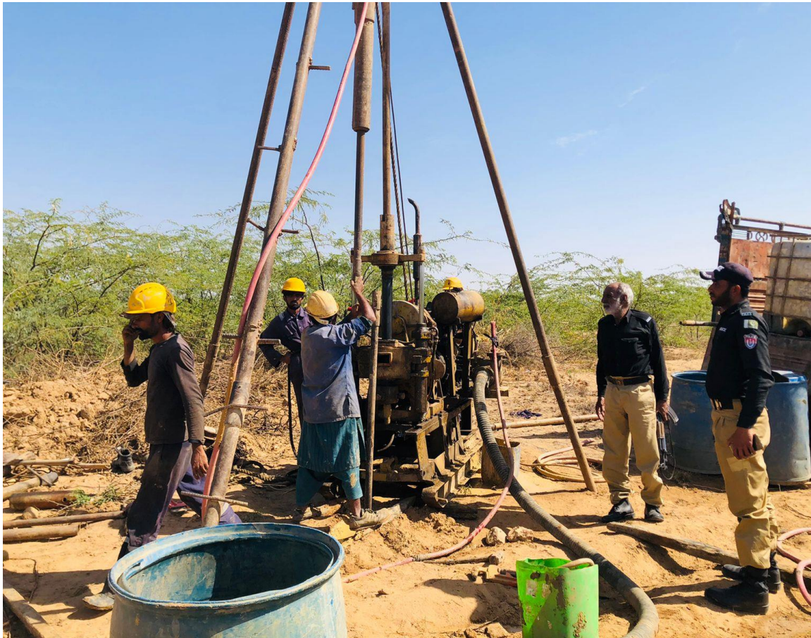
Figure A-2: Performance of standard penetration test
