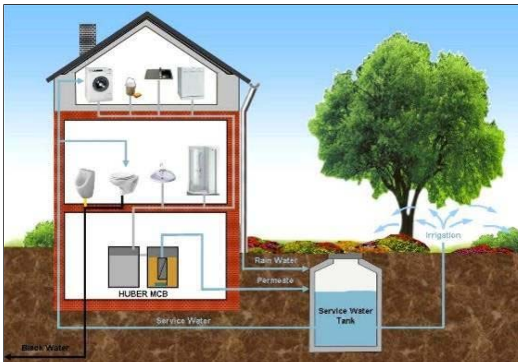
Figure 36: Grey Water Collection & Recycle Process
